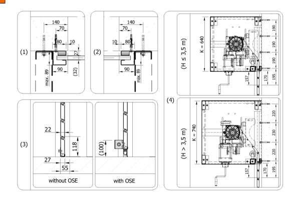
**Minimum required dimensions of steel structure**
