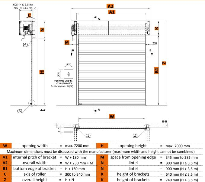
Average weight of slats with filling (RGS 22V, EW 120) =  $23.5 \text{ kg/m}^2$ Average weight of slats without filling (RGS 22, EW 45) =  $21.9 \text{ kg/m}^2$
