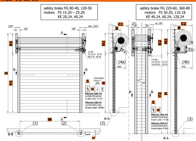
\* - for gates with W  $\geq$  6 m the marked dimensions are 45 mm bigger
