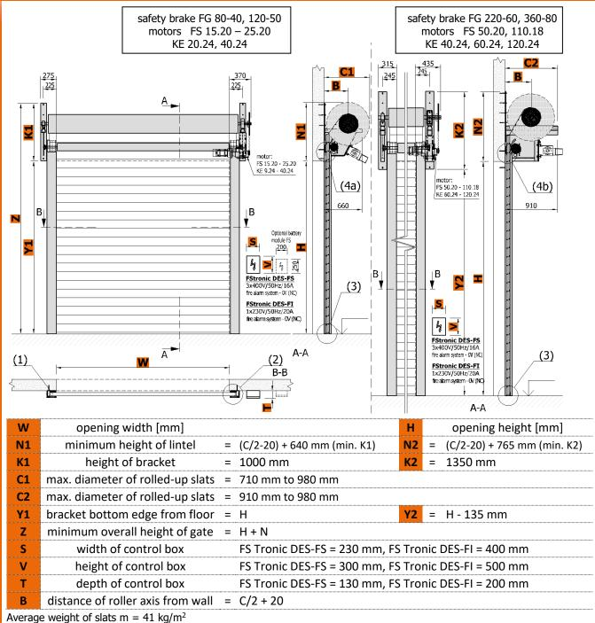
Average weight of main roller with connection slats m = 70 kg/m
